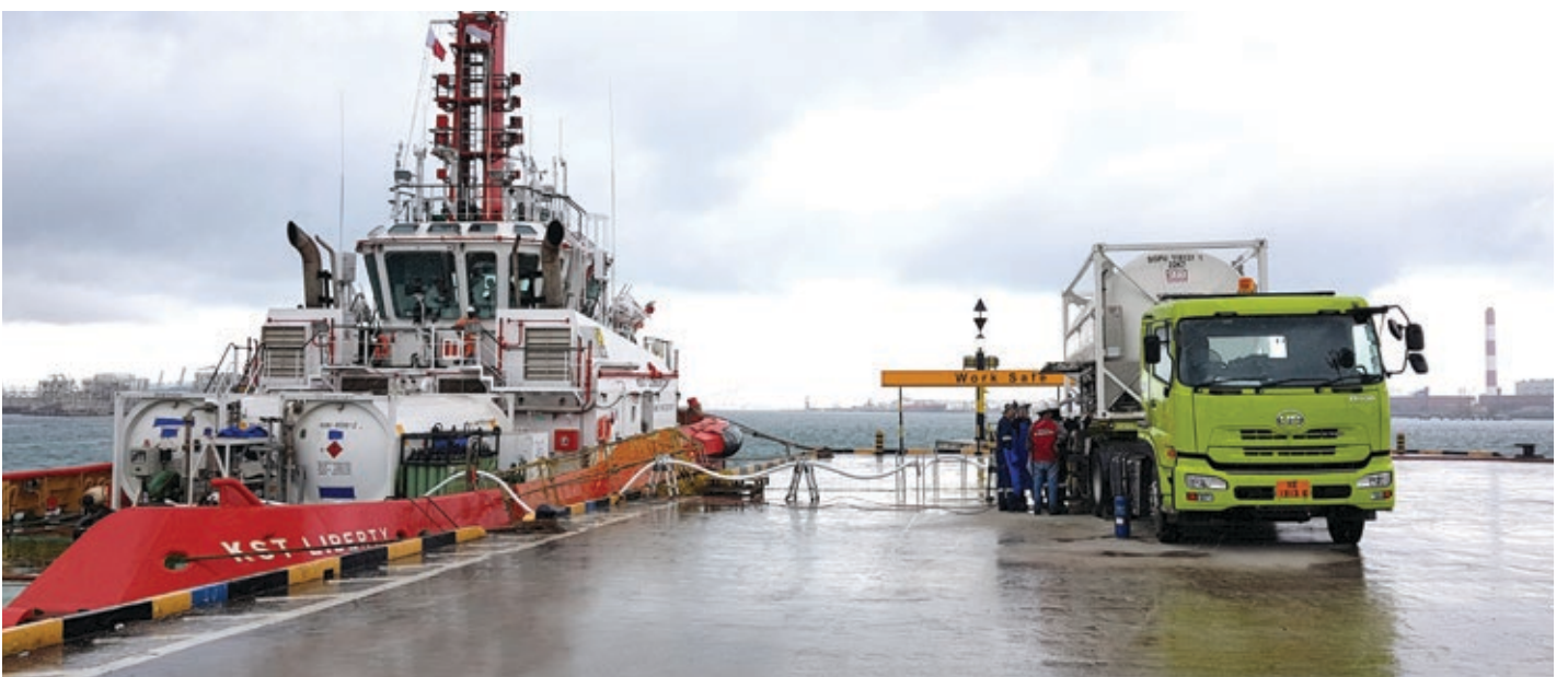
LNG Transferring and Bunkering Service - The 1st LNG-powered tug project Southeast Asia
